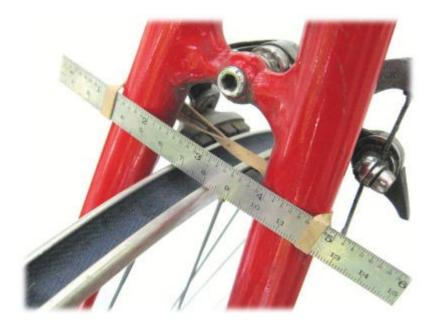
Remove the tire from the wheel. Place the wheel back onto the bike. Attach a ruler to the frame with a rubber band or painters tape. Give the wheel a slow spin and proceed to True the wheel as described earlier in the document. Tighten or loosen each spoke to remove unwanted wobble, hop and dish.
