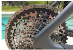
XPLR is a 10-44T 12 speed, narrow/wide 1x chainring with either a 38T or 46T, to give you a 440% range. The 6 high range gears on the cassette are closely spaced like a road bike, while the low range gears have a wider spacing to get you up those steep climbs and through the rough terrain. (10-11-13-15-17-19-21-24-28-32-38-44) The SRAM 12s cassettes utilize the XDR Freehub bodies and the SRAM flattop chain that have slightly larger roller diameters.
