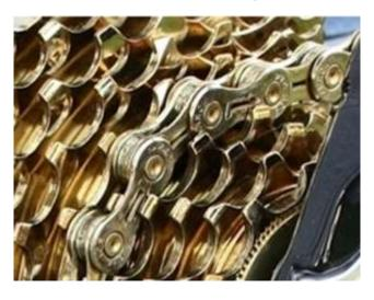
A new chain usually comes in a longer length than you'll need. Therefore you'll need to determine the correct length for your bike, then "break" the chain. Don't worry, we're not actually going to break the chain. That's just a term used to describe the action of shortening a chain by
