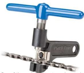
The chains length is changed by pushing one of the pins out. For this you'll need a special tool seen here. It should be noted that the pins of a chain are riveted onto the chain plates. Once removed, you can never use that pin again. The best way to determine the length of your new chain is to make it the same length as the old chain! Don't forget to install a Quick Link®.
