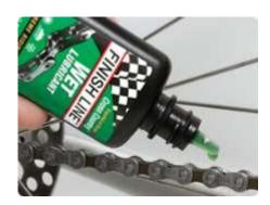
Make sure each and every roller receives a drop of lubricant. Spin the crank around for about a minute, then wipe off the excess lube from the outside of the chain. Dry lubricant goes on wet, but the carrier solution will soon evaporate leaving the chain dry. A wet lubricant can be oil based or synthetic, and will remain wet.
